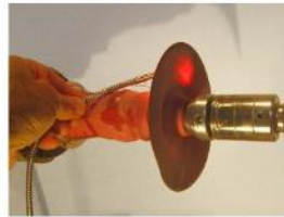
Checking wall thickness with light
