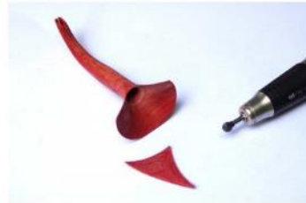
Gusset made to fit front of spout
