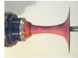
Laser dot showing extent of hollowing
